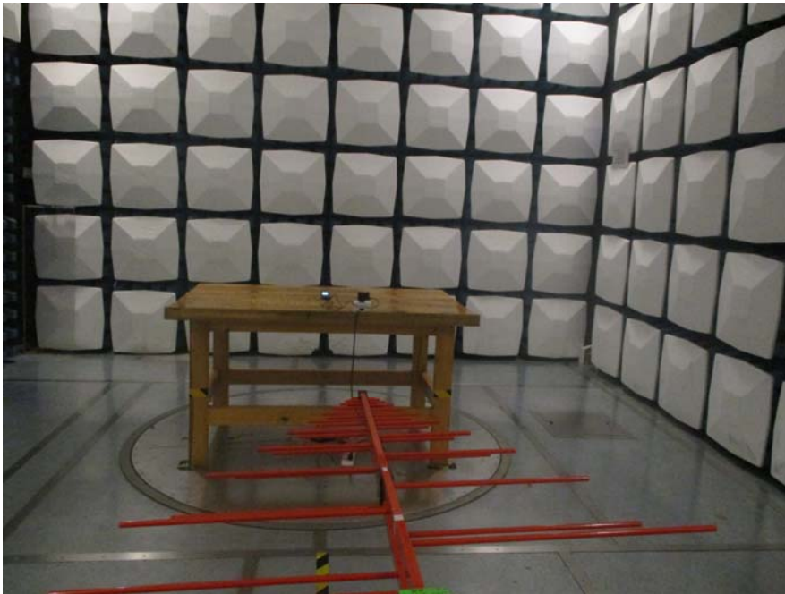
Radiated Emission View (Above 1GHz)
