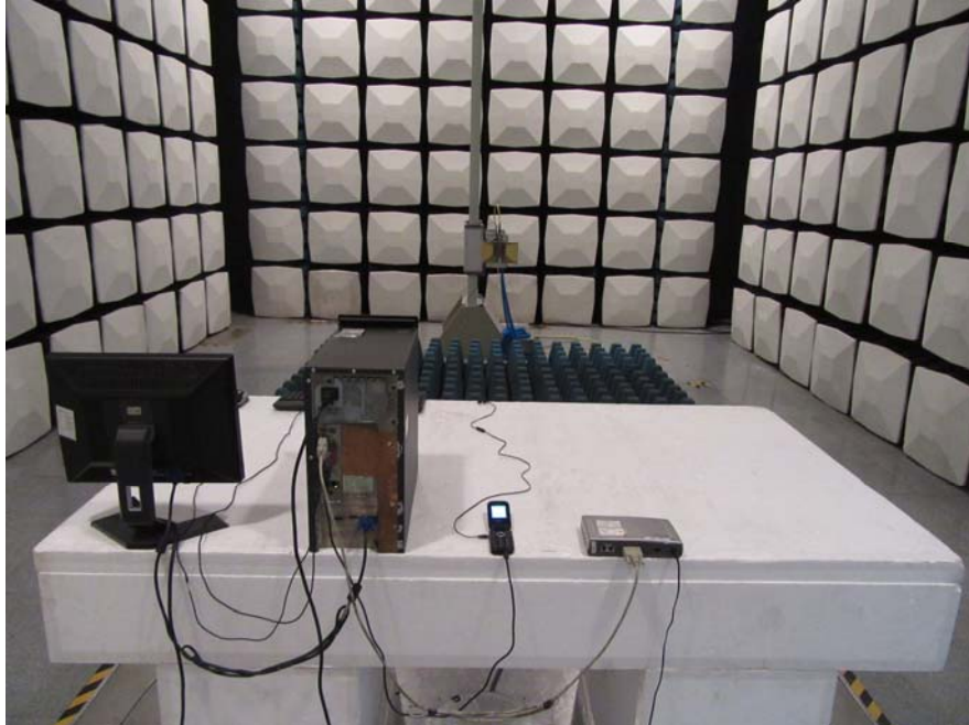
Radiated Emission - Rear View (Above 1 GHz)
