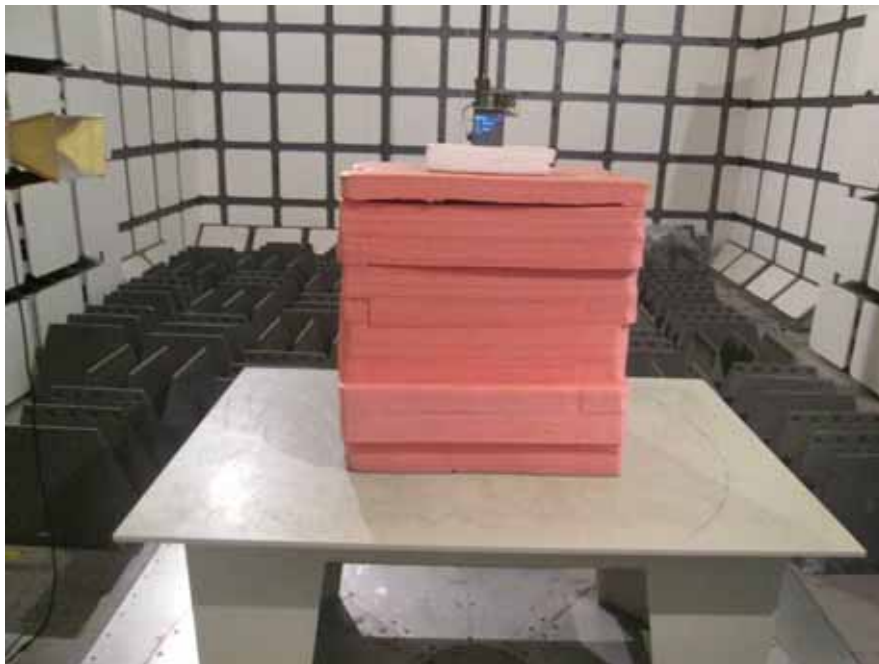
Radiated Emissions Test View (Above 1 GHz)
