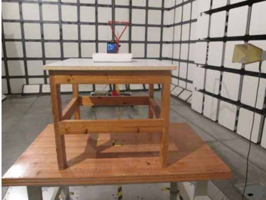
Radiated Emissions Test View (Below 1 GHz)
