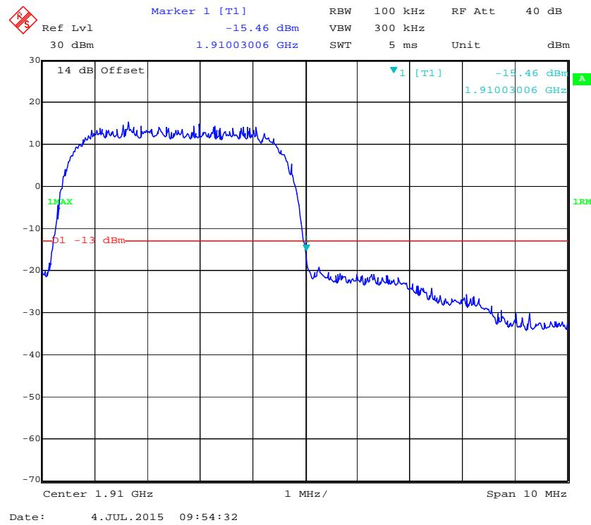
**PCS Band, Left Band Edge for HSDPA (16QAM) Mode**
