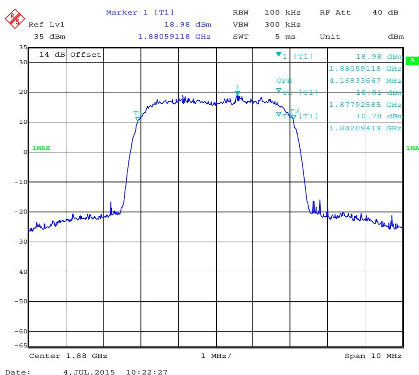
**26 dB Emissions Bandwidth for HSUPA (BPSK) Mode**
