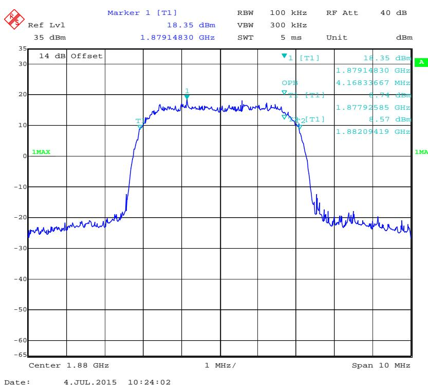
**26 dB Emissions Bandwidth for EDGE Mode**
