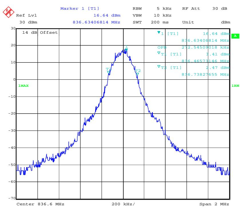
**PCS Band (Part 24E)****26 dB Emissions Bandwidth for GSM (GMSK) Mode**
