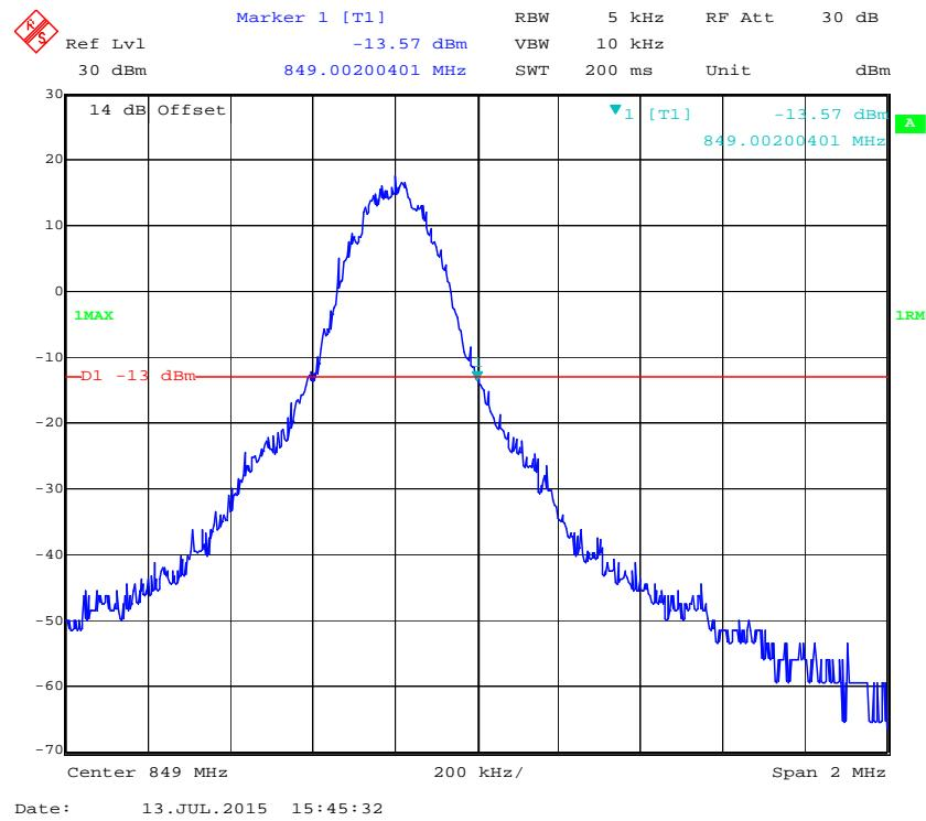
**PCS Band, Left Band Edge for GSM (GMSK) Mode**
