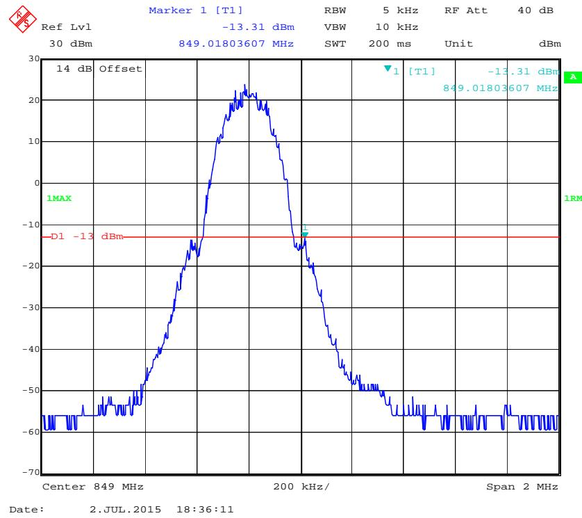
**Cellular Band, Left Band Edge for WCDMA (BPSK) Mode**
