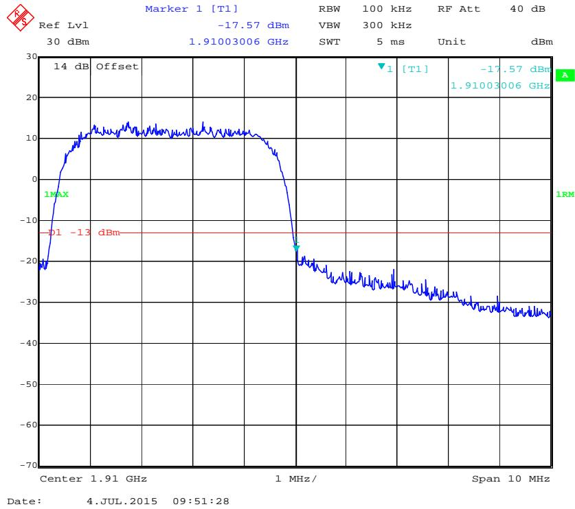
**PCS Band, Left Band Edge for HSUPA (BPSK) Mode**
