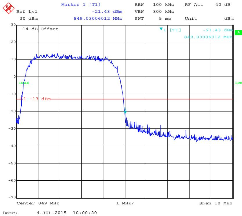
**Cellular Band, Left Band Edge for HSUPA (BPSK) Mode**
