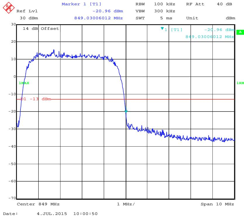
**Cellular Band, Left Band Edge for HSDPA (16QAM) Mode**
