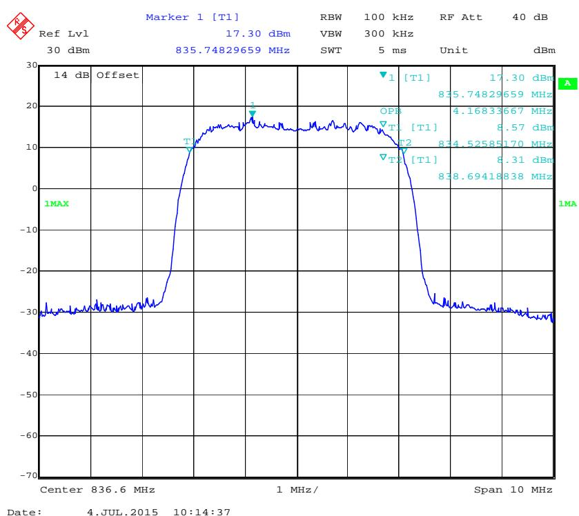
**26 dB Emissions Bandwidth for HSUPA (BPSK) Mode**
