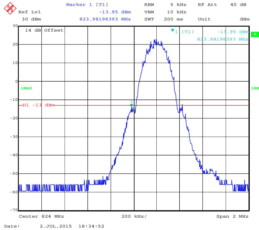
**Cellular Band, Right Band Edge for GSM (GMSK) Mode**
