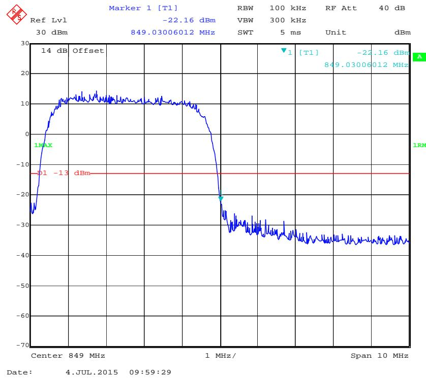
**Cellular Band, Left Band Edge for EDGE Mode**
