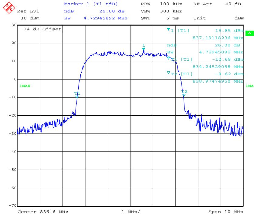
**99% Occupied Bandwidth for HSUPA (BPSK) Mode**
