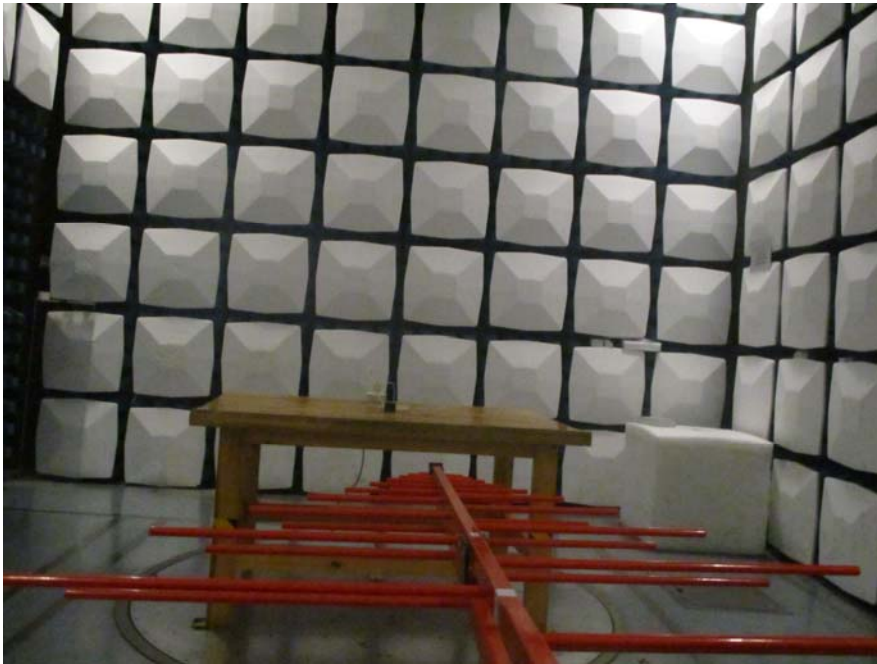
Radiated Emission View (Below 1GHz)
