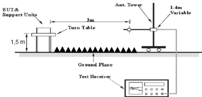
The radiated emission Below 1GHz tests were performed in the 3 meters chamber test site, above 1GHz tests were performed in the 3 meters chamber test site, using the setup accordance with the ANSI C63.10-2013. The specification used was the FCC 15.209, and FCC 15.247 limits.
