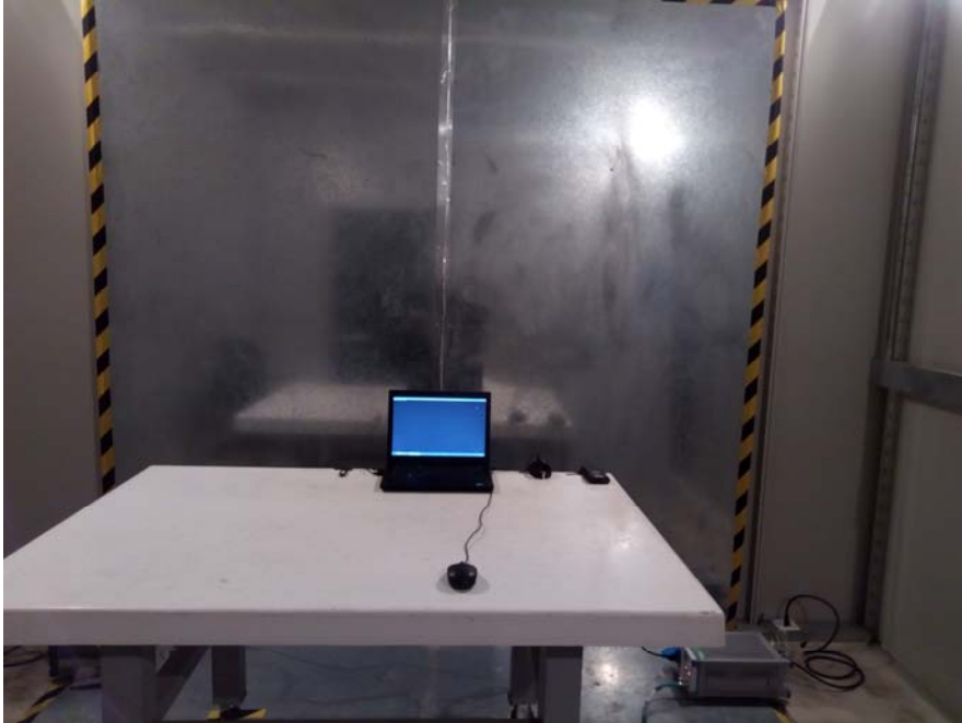
Conducted Emissions - Front View
