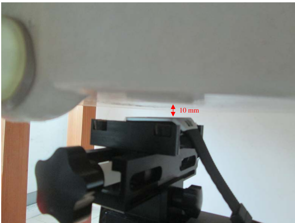
Face up Setup Photo (10 mm)
