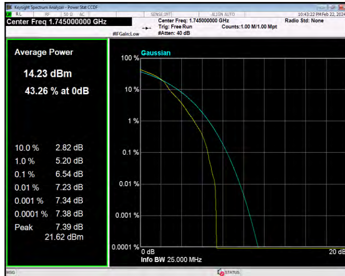
Band66 16QAM BW=15MHz Channel=132597 RB Size=1 Position=#0
