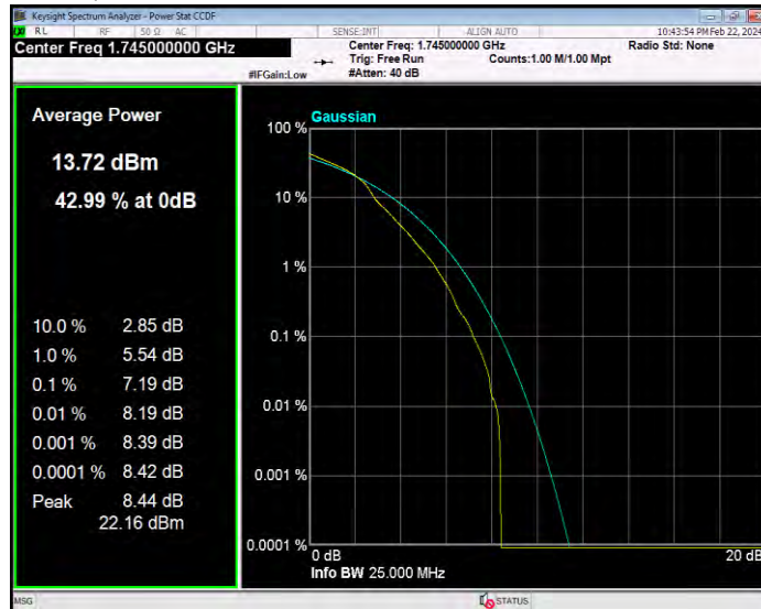
Band66 16QAM BW=20MHz Channel=132572 RB Size=1 Position=#0
