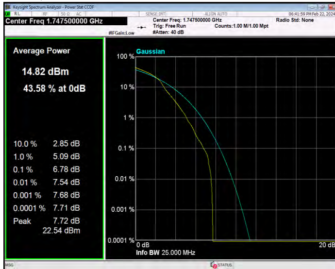
Band4 16QAM BW=15MHz Channel=20325 RB Size=1 Position=#0
