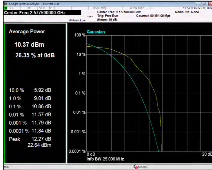
Band38 16QAM BW=15MHz Channel=38000 RB Size=1 Position=#0
