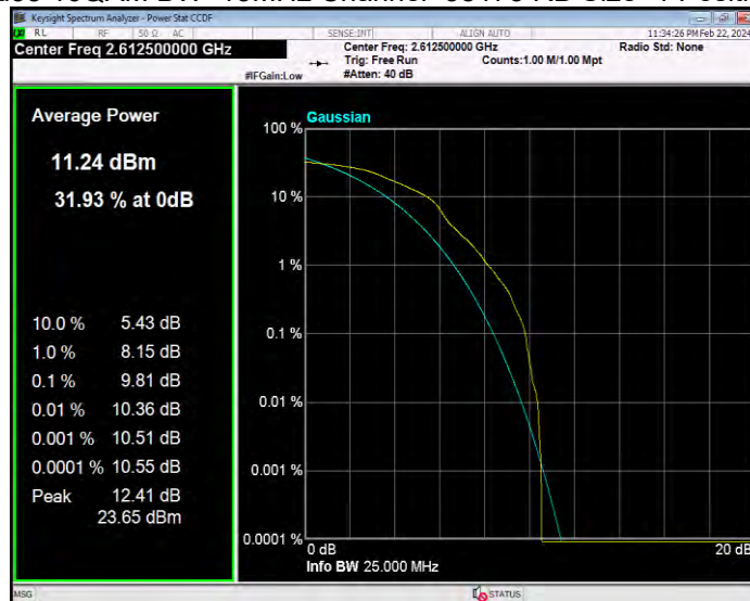
Band38 16QAM BW=15MHz Channel=38175 RB Size=1 Position=#0
