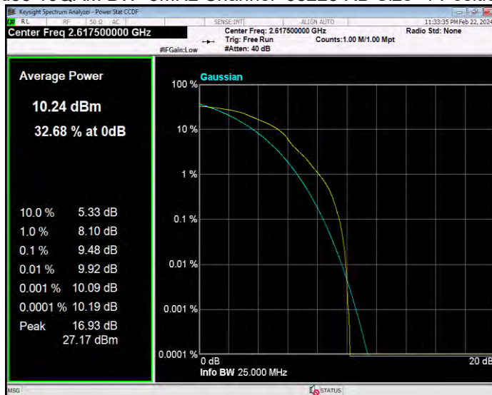
Band38 16QAM BW=5MHz Channel=38225 RB Size=1 Position=#0
