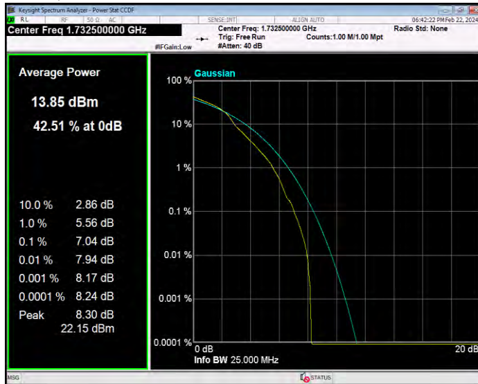
Band4 16QAM BW=20MHz Channel=20300 RB Size=1 Position=#0
