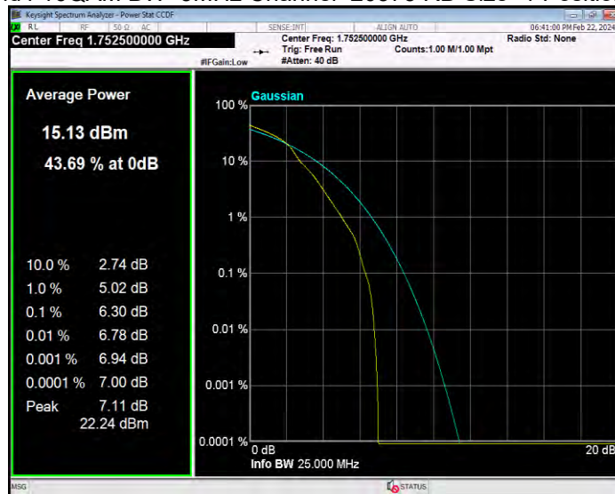
Band4 16QAM BW=5MHz Channel=20375 RB Size=1 Position=#0
