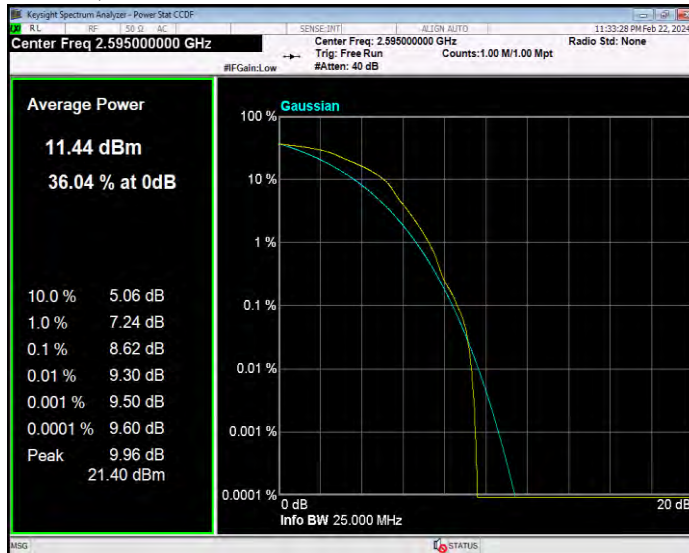
Band38 16QAM BW=5MHz Channel=38225 RB Size=1 Position=#0
