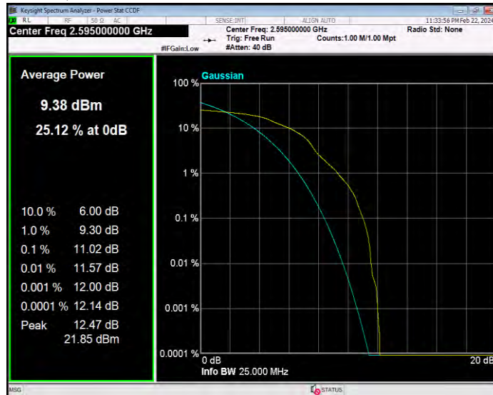
Band38 16QAM BW=10MHz Channel=38200 RB Size=1 Position=#0
