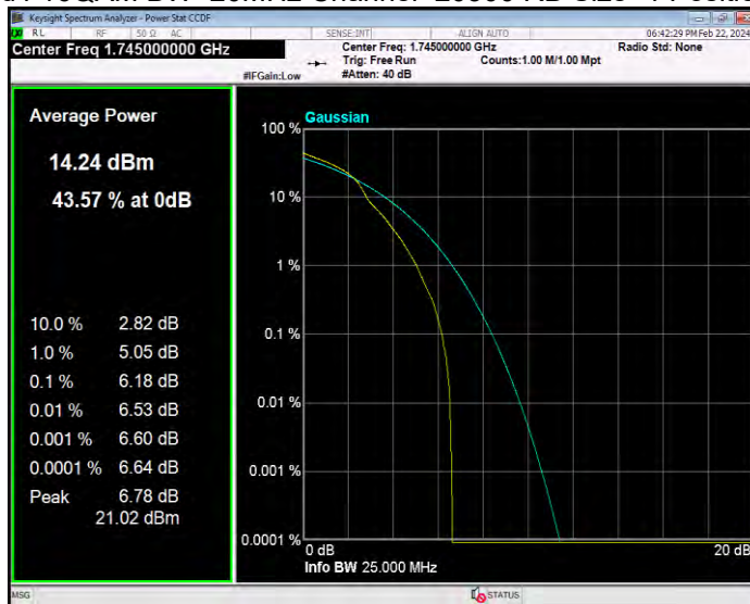
Band4 16QAM BW=20MHz Channel=20300 RB Size=1 Position=#0
