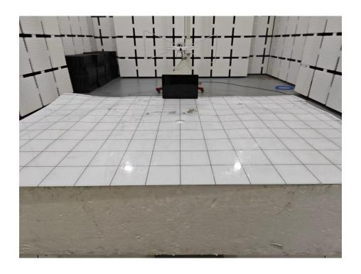
Set-up for Radiated Spurious Emission, Above 1GHz
