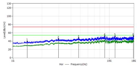
Frequency Factor Reading Level Limit Margin No. Detector Polar MHz dBuVdB/m dBuV/m dBuV/m dΒ 1\* 1405.9000 60.65 -21.44 39.21 74.00 -34.79 PK Hor 2\* 2963.5000 54.02 -8.95 45.07 74.00 -28.93 PΚ Hor 3\* 54.65 4808.0000 -6.81 47.84 74.00 -26.16 PK Hor 4\* PK 9000.6000 55.82 -3.67 52.15 74.00 -21.85 Hor 11495.4000 5\* 53.45 -1.83 51.62 74.00 -22.38 PΚ Hor 6\* 17817.2000 50.20 1.94 52.14 74.00 -21.86 PΚ Hor
