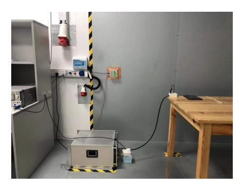
Set-up for Radiated Emission (RE), Below 1GHz
