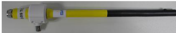
Figure 1 – Satimo COMOHAC T-coil Probe
