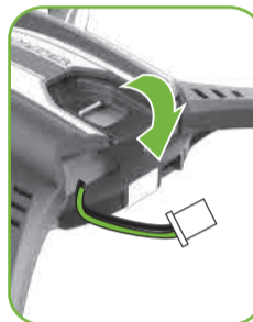
Close the battery latch
