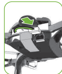
Connect the battery
