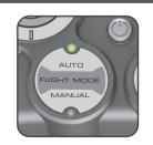
MANUAL mode is better for experienced pilots. When the left thumbstick is pushed all the way up the drone will spin its motors as fast as it can while maintaining stability, and when the left thumbstick is pushed all the way down the motors will stop spinning completely.
