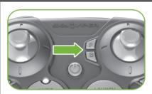
IF THE DRONE DRIFTS FORWARD: Press "B" button several times until the drone stops drifting forward
