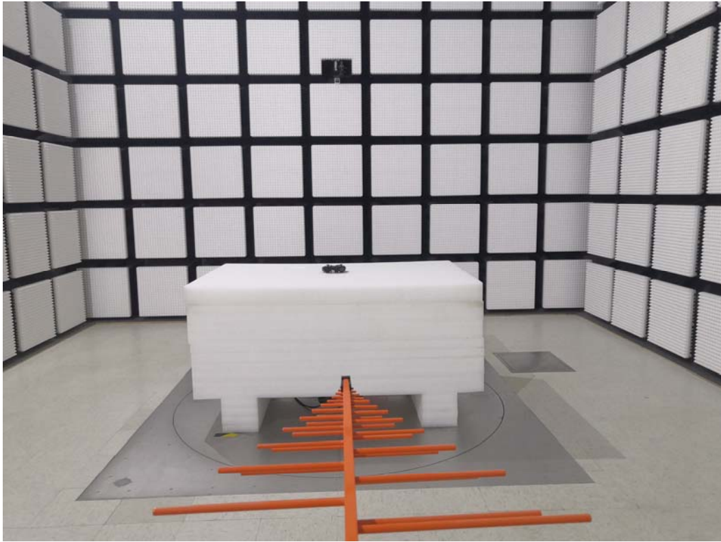
Radiated Emission Above 1GHz View
