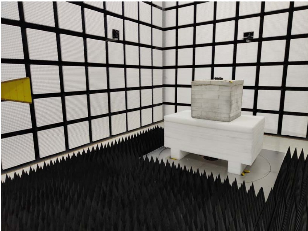
Radiated Emission Above 1GHz View
