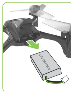
Remove LiPo battery from compartment and unplug cable
