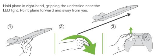
Toss and release plane slightly up and forward, then immediately push *throttle forward full* to complete launch.
