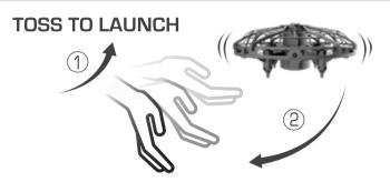
Turn drone on and hold it upright in front of you in the palm of your hand. Keep drone level and give it a slight toss upward, then drop your hand quickly downward. Drone will automatically start to fly. Toss drone high to hover high, toss drone low to hover low.
