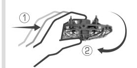
Quickly grab drone and flip upside down to stop. If out of reach, blast drone to make it fall or wait until battery power is depleted. Drone will auto-land itself.
