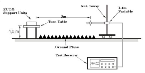
The radiated emission below 1GHz tests were performed in the 10 meters chamber test site, above 1GHz tests were performed in the 3 meters chamber test site B, using the setup accordance with the ANSI C63.10-2013. The specification used was the FCC 15.209, and FCC 15.249 limits.
