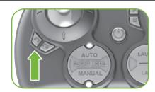
IF THE DRONE SPINS COUNTER-CLOCK-WISE (VIEWED FROM ABOVE): Press the 🔼 button several times until the drone stops
