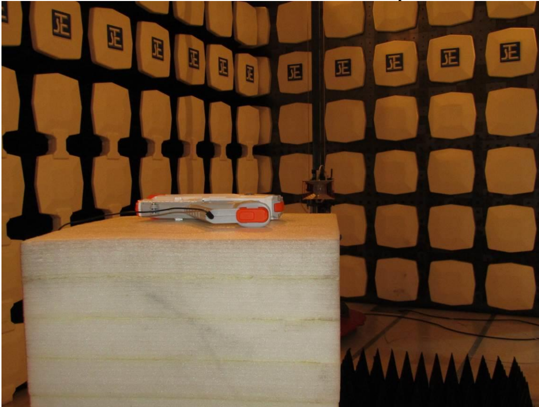
Measurement of Radiated Emission Test Set Up
