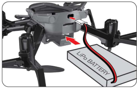
Insert fully charged LiPo battery into the underside of drone, then connect the battery to back of the drone.
