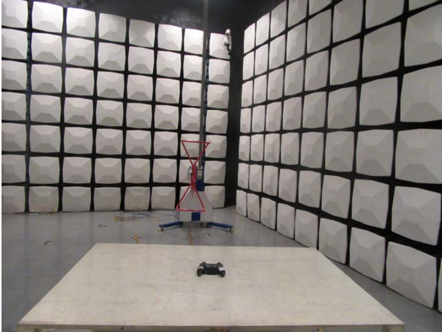
Radiated Emission View (Below 1GHz)
