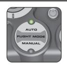
MANUAL mode is better for experienced pilots. When the left thumbstick is pushed all the way up the drone will spin its motors as fast as it can while maintaining stability, and when the left thumbstick is pushed all the way down the motors will stop spinning completely.
