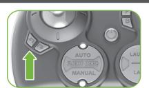
IF THE DRONE SPINS COUNTER-CLOCK-WISE (VIEWED FROM ABOVE): Press the button several times until the drone stops spinning.
