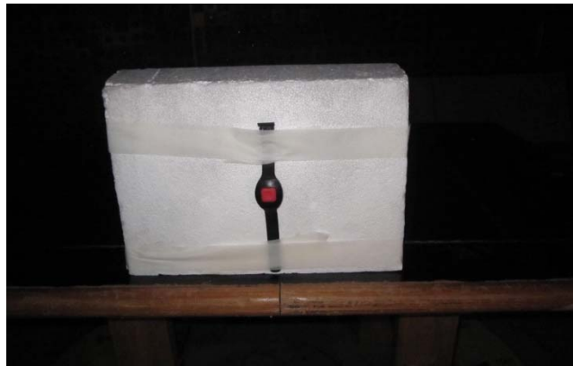
Photograph 6.4.3 EUT in Z-axis orthogonal position
