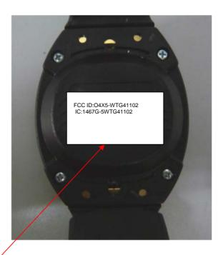
Label with FCC ID:04X5-WTG41102 and IC:1467G-5WTG41102 is located at the rear side panel of the Wrist tag. The statement according to FCC part 15 §15.19(a)(3) is placed in User's Guide, page 4 (Application exhibit User\_manual\_26769).
