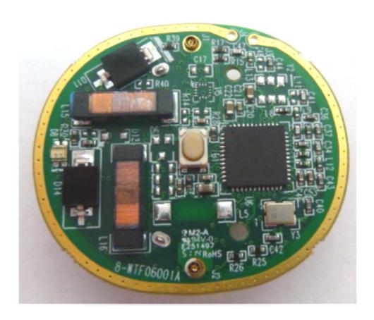
Photograph No.4 Tag PCB second side view (model 5-WTG41102-0)
