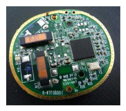
Photograph No.5 Tag PCB second side view (model 5-WTG40002-0)
