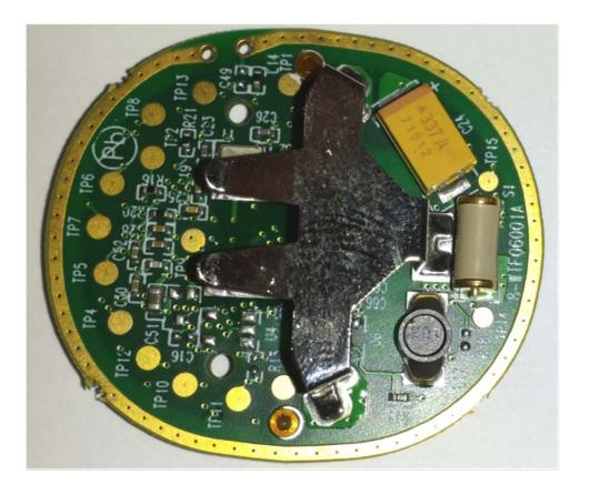
Photograph No.3 Tag PCB front view with shield removed
