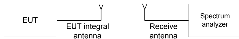
Figure 7.1.1 Setup for transmitter shut down test
