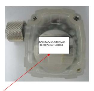
Label with FCC ID:04X5-STC00433 and IC:1467G-5STC00433 is located at the rear side panel of the temperature sensor. The statement according to FCC part 15 §15.19(a)(3) is placed in User's Manual, page 5 (Application exhibit 5-STC\_UserMan).
