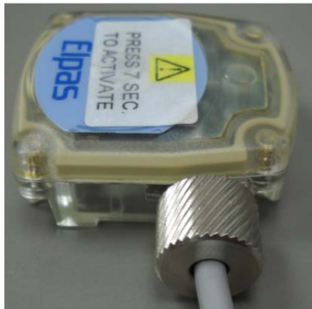
Photograph 6.4.3 EUT in Z-axis orthogonal position
