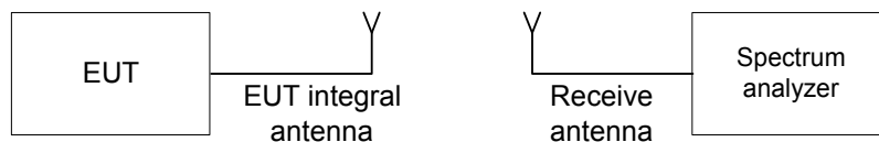
Figure 7.1.1 Setup for transmitter shut down test
