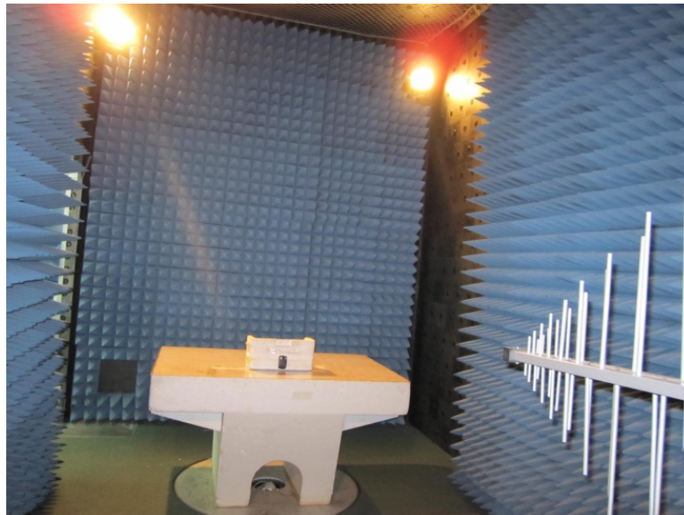
Photograph 8.1.1 Setup for final radiated emission measurements
