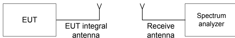
Figure 7.1.1 Setup for transmitter shut down test
