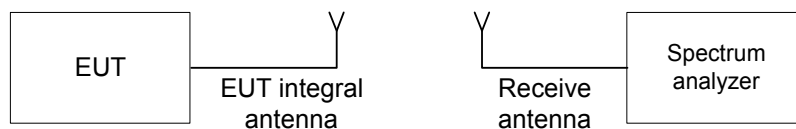
Figure 7.1.1 Setup for transmitter shut down test
