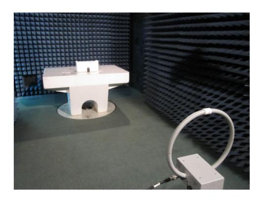
Photograph No.2 Setup for spurious emission field strength measurements in the anechoic chamber, EUT close view
