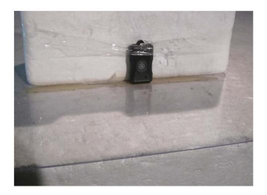
${\bf Photograph~No.3}$  Setup for carrier field strength, spurious emission field strength measurements in the anechoic chamber in 30 – 1000 MHz range
