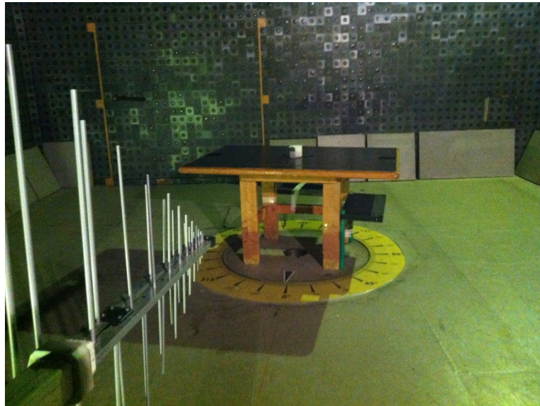
Photograph 8.1.1 Setup for radiated emission measurements
