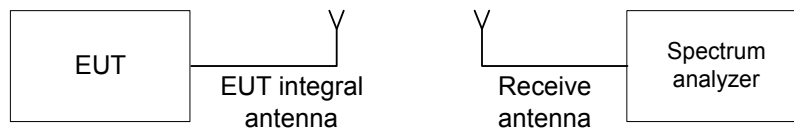
Figure 7.1.1 Setup for transmitter shut down test
