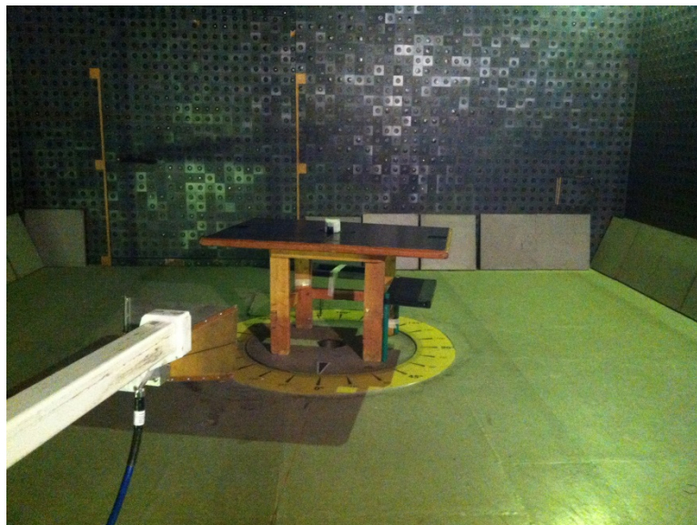
Photograph 8.1.2 Setup for radiated emission measurements
