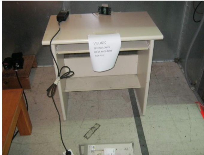
Figure 2. Conducted Emission From AC Mains Test
