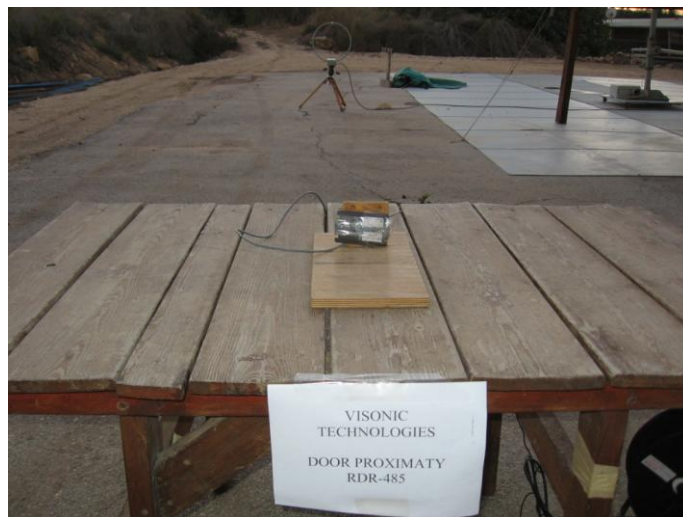
Figure 3. Radiated Emission Test
