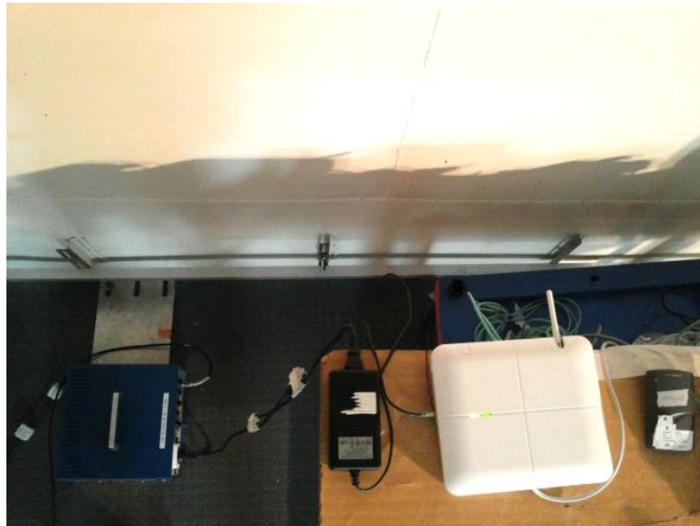
Photograph 8.1.1 Setup for conducted emission measurements
