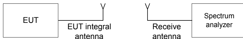
Figure 7.1.1 Setup for transmitter shut down test
