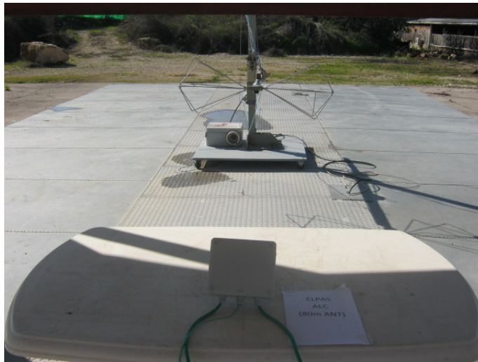
Figure 10. Radiated Emission Test - 5-ALC11123-0 80m antenna
