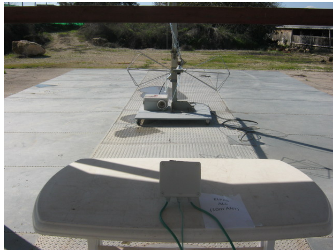
Figure 8. Radiated Emission Test - 5-ALC11123-0 10m antenna
