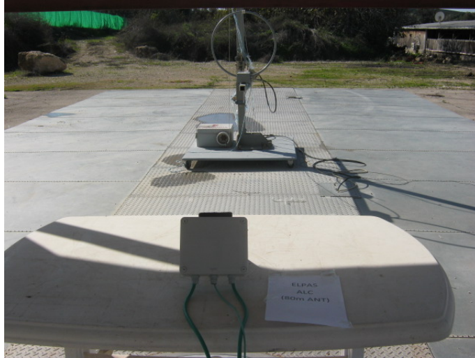
Figure 9. Radiated Emission Test - 5-ALC11123-0 80m antenna
