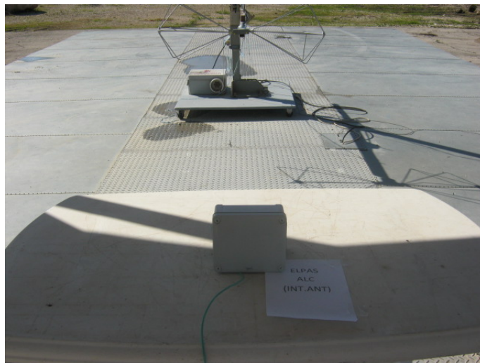
Figure 6. Radiated Emission Test - 5-ALC11122-0
