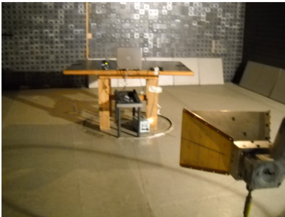
Photograph No.3 Setup for spurious emission field strength measurements in the anechoic chamber above 1 GHz
