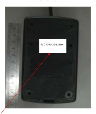
Label with FCC ID:04x3-63290 is located at the rear side panel of the RDR-PXT proximity reader. The statement according to FCC part 15 §15.19(a)(3) is placed in Installation Guide, page 2 (Application exhibit RDR-PXT\_UserMan).
