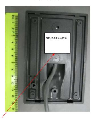
Label with FCC ID:04X3-63210 is located at the rear side panel of the RDK-4 proximity reader. The statement according to FCC part 15 §15.19(a)(3) is placed in Installation Guide, page 2 (Application exhibit RDK-4\_UserMan).
