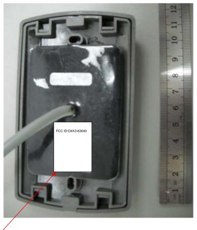
Label with FCC ID:O4X3-63040 is located at the rear side of the RDR-2 proximity reader. The statement according to FCC part 15 §15.19(a)(3) is placed in Installation Guide, page 2 (Application exhibit RDR-2\_UserMan).
