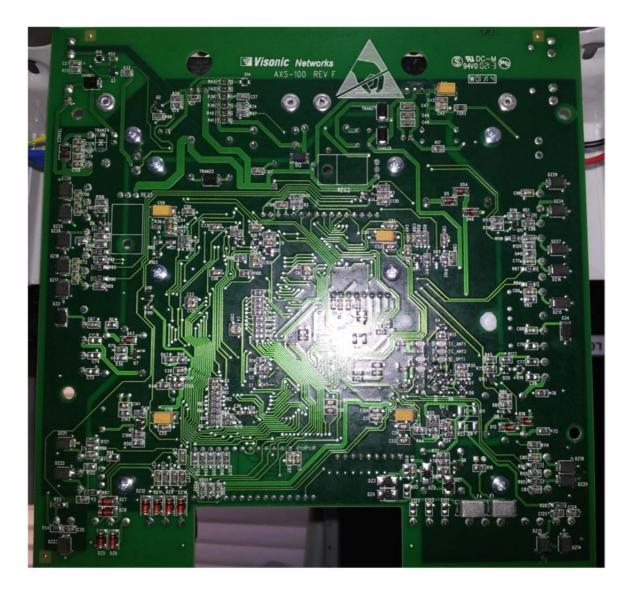
Photograph No.3 AXS-100 control panel main PCB second side view
