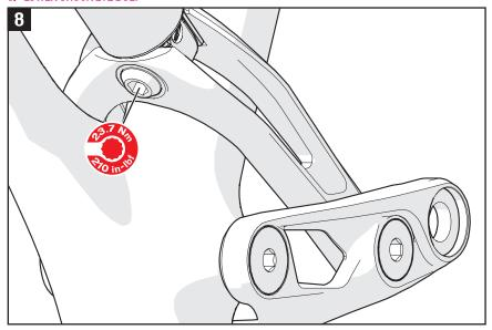
■ Once all pivot locations are assembled and torqued to specification, torque the lower shock eye bolt.
