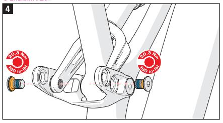
■ Align the extension with the bearings, then insert the pivot bolts.
