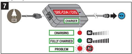
During the charging process, the diode on the charger will glow red (fig.7). When the battery is fully charged, the diode on the charger will turn green.
