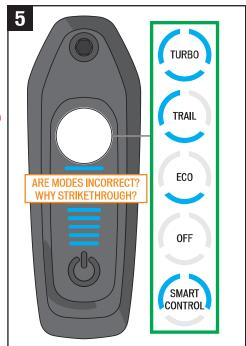
To switch into a different support mode, press the + or - button on the top tube display battery, Mission Control app or LEV display unit computer. On the remote, after reaching the strongest or weakest mode, the system will not continue to switch. To reduce from TURBO to TRAIL to ECO, you have to press the - button. To increase from ECO to TRAIL to TURBO, you have to press the + button.
