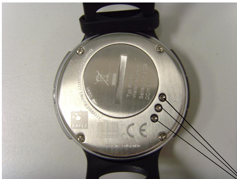
The pins for connecting the USB cable
