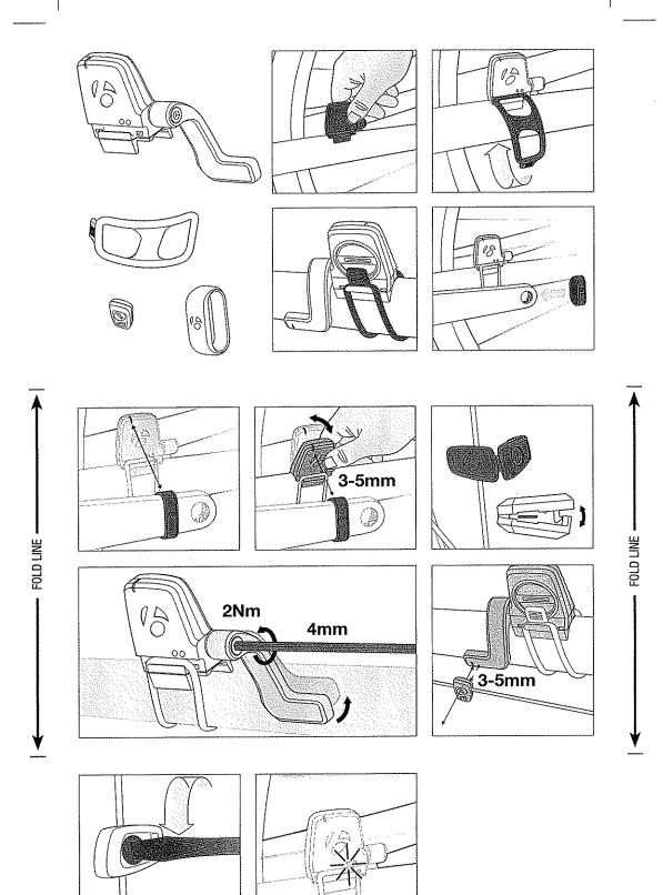
Red LED will flash when the speed magnet is lined up correctly. Green LED will flash when the cadence magnet is lined up correctly. LEDs will only flash for the first ten revolutions.
