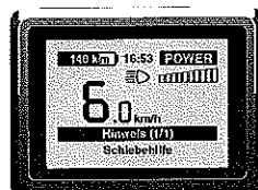
Impulse Evo (Smart) display: Push assist activated
