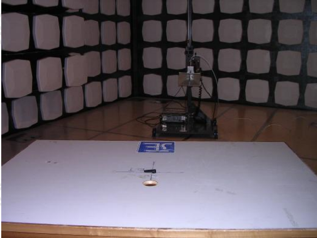
Measurement of Radiated Emission Test Set Up
